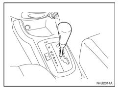
Movement between certain positions requires pushing the shift lever to the passenger side while shifting. This prevents you from changing positions unexpectedly by blocking the straight movement of the shift lever when the vehicle is moving.
